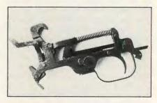
ABOVE: Type 63 trigger mechanism is another copy of the M1 Garand's. This left-side view shows the disassembly lever.
